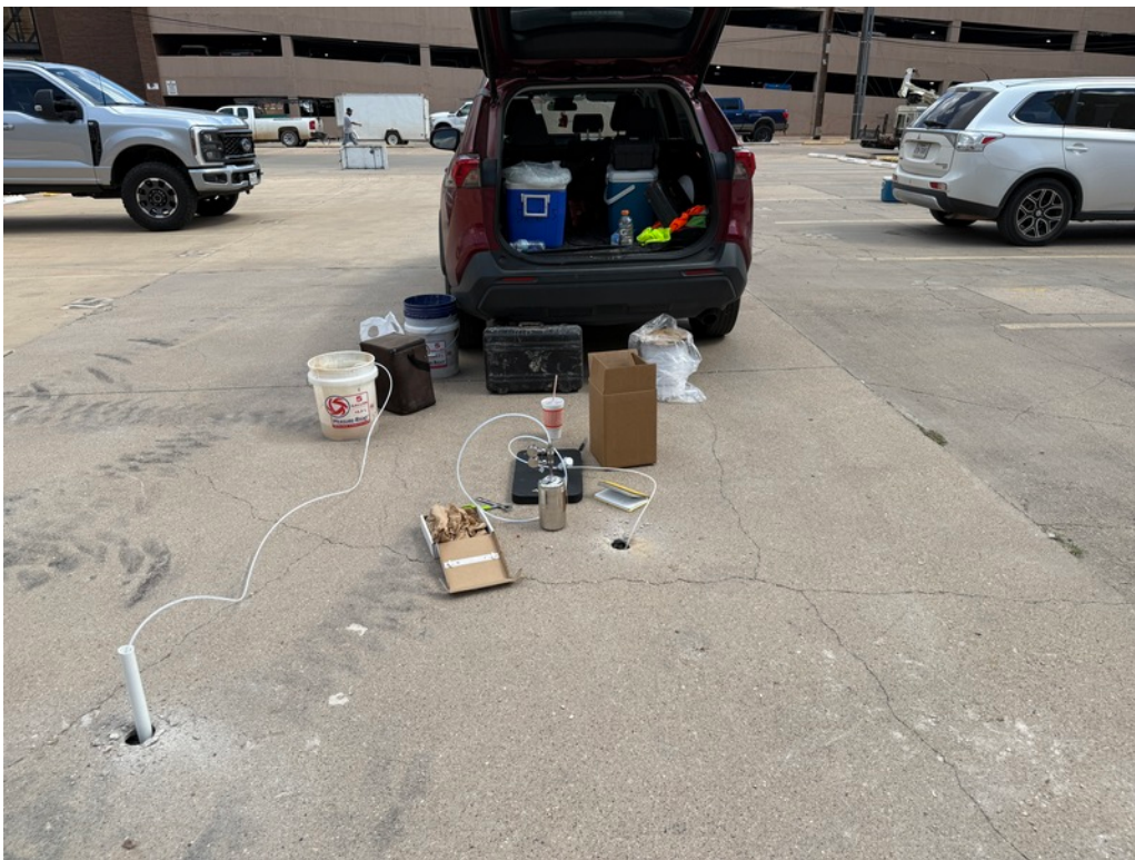
10. (44) View east of TMW-5 groundwater purging activities
